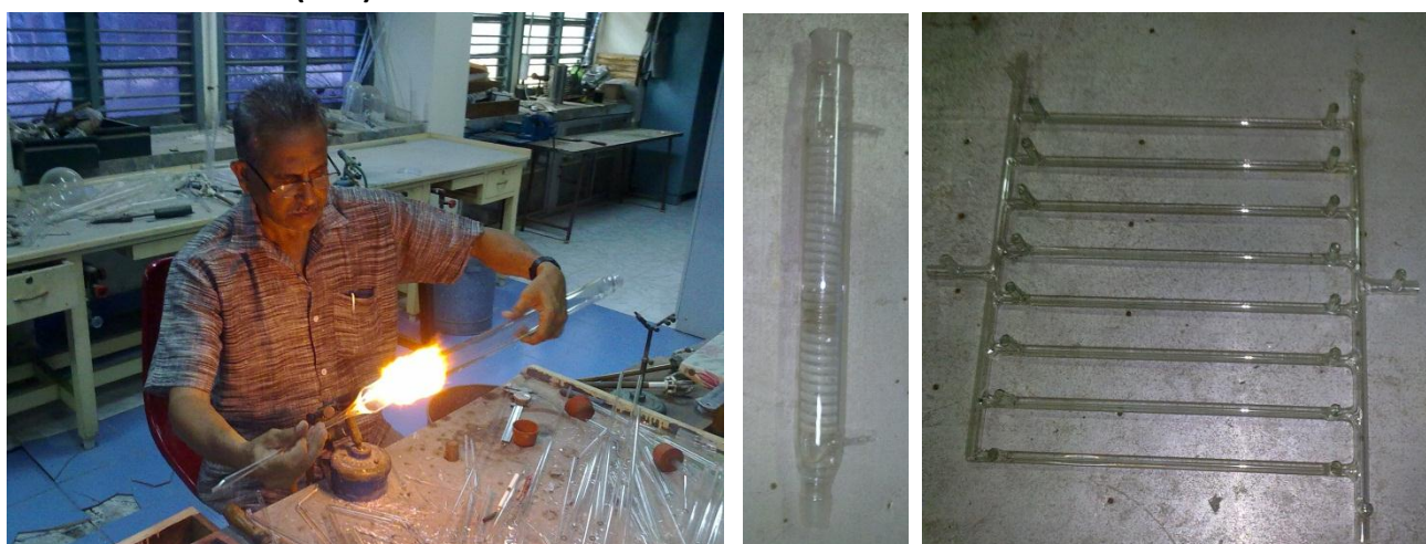
From left to right. Mr Narasingh working in full concentration. A coil condenser. Setup to study the two-phase flow distribution in minichannel arrays.
